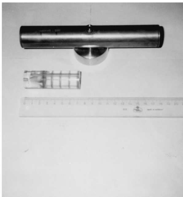
Fig. 3. Photograph of the separation chamber, with a 0.5-ml volume and a rotor with a diameter of 18 cm, of the laboratory-made elutriator described in Ref. [70]. The rotor may be mounted on a benchtop centrifuge.
